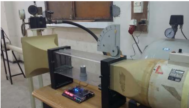
Fig.6. Wind tunnel calibration of the hot wire sensor.
