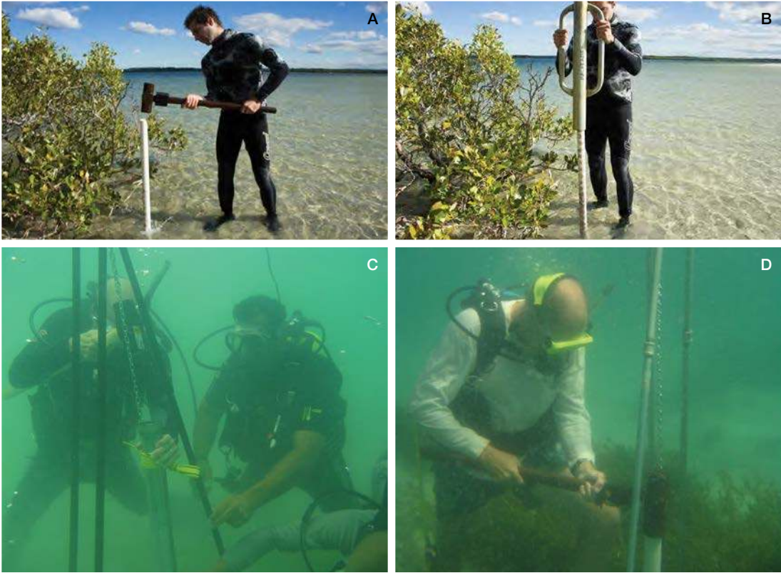
Figure 3.7 A demonstration of method used to drive corer into soil in seagrass meadows. (A) Shallow water with a sledgehammer (© Sarah Hoyt, CI), (B) shallow water with a post-pounder (© Sarah Hoyt, CI), (C and D) deep water with a sledgehammer (© James Fourqurean, FIU)
