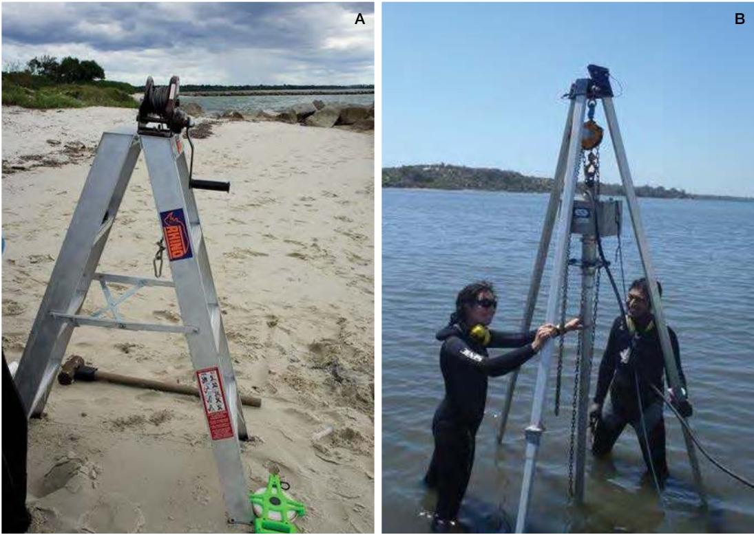
Figure 3.8 Set up for core sampling in seagrass ecosystems. Instruments for seagrass soil coring: (A) ladder with crank for removing coring device from soft soil in shallow water (© Sarah Hoyt, CI), (B) sturdy tripod with weighted pulley system for removing coring device from soft soil in either shallow or deep water (© Oscar Serrano, ECU)
