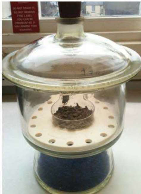
Figure 3.18 Soil sample cooling to room temperature in desiccator (© Hillary Kennedy, UWB)
