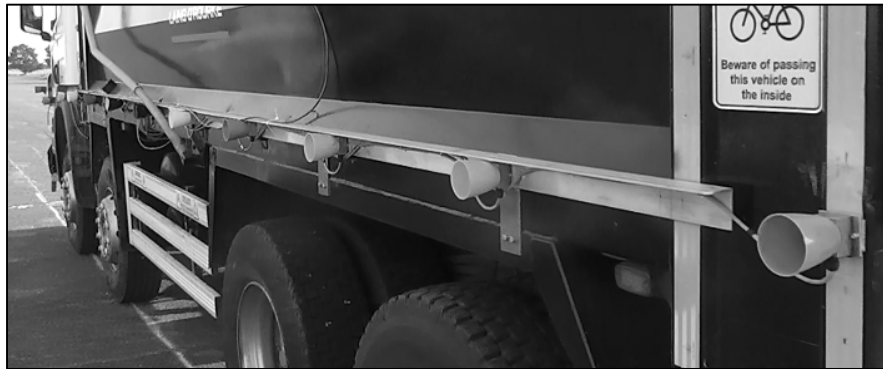
Fig. 6. Ultrasonic sensors mounted along the side of the test vehicle
