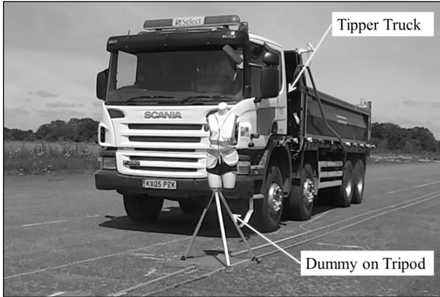
Fig. 5. Testing setup showing the truck & the dummy cyclist
