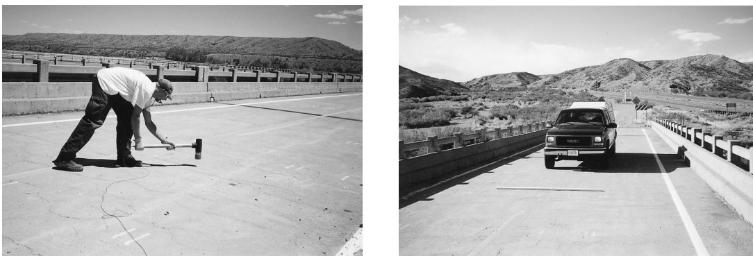
Figure 6: Methods of forced excitation of the Alamosa Canyon Bridge; (left) modal hammer and (right) flatbed truck driving over a wood stud place in the center of the span
