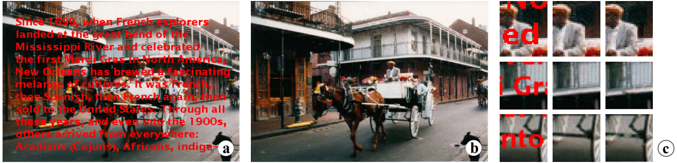
Figure 6. Inpainting with a Field of Experts. (a) Original image with overlaid text. (b) Inpainting result from diffusion using the FoE prior. (c) Close-up comparison between a (left), b (middle), and the results from [3] (right).
