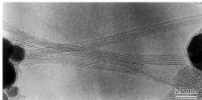
Fig. 10. TEM image of long bundles of single-walled nanotubes (SWNT) obtained when a high purity carbon anode was doped with Ni.
