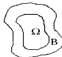
Fig. 2. Region to be filled-in and corresponding surrounding band from where the information is considered.
