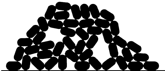
Figure B1. A pile of particles with an increased volume due to the presence of two pores caused by particle bridging. [After German PCC]
