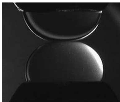
Fig. 6 Two interacting glycerol drops in silicone oil that have emerged from two opposing capillaries.
