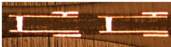
Fig. 1 Cross section of ultra thin RXP substrate
