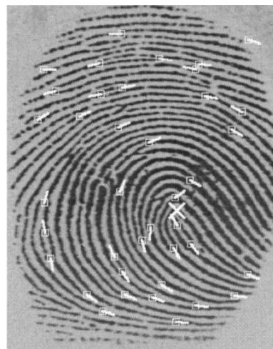
Fig. 1. Ridges and automatically detected minutiae points in a fingerprint image. The core is marked with a \times .
