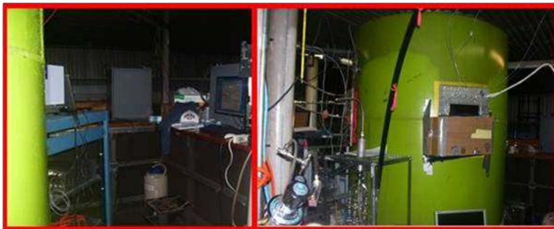
Figure 3.4 New Matrix FTIR spectrometer is shown atop the blue table and coupled to the FSL chimney (left frame) with the D-mirrors on opposite side of the chimney (right frame, behind cardboard piece).
