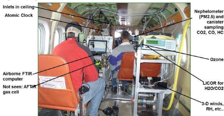
Figure 7.3 Photograph of the AFTIR system installed in the Twin Otter for Lejeune campaign. Other equipment is as indicated, along with scientists Ian Burling and Shawn Urbanski.
