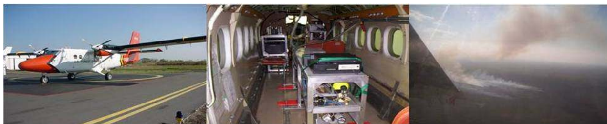
Figure 2.5 Left: the USFS Twin Otter aircraft. Center: the infrared spectrometer system and PM instruments in cabin. Right: view from Twin Otter just before entering a smoke plume.
