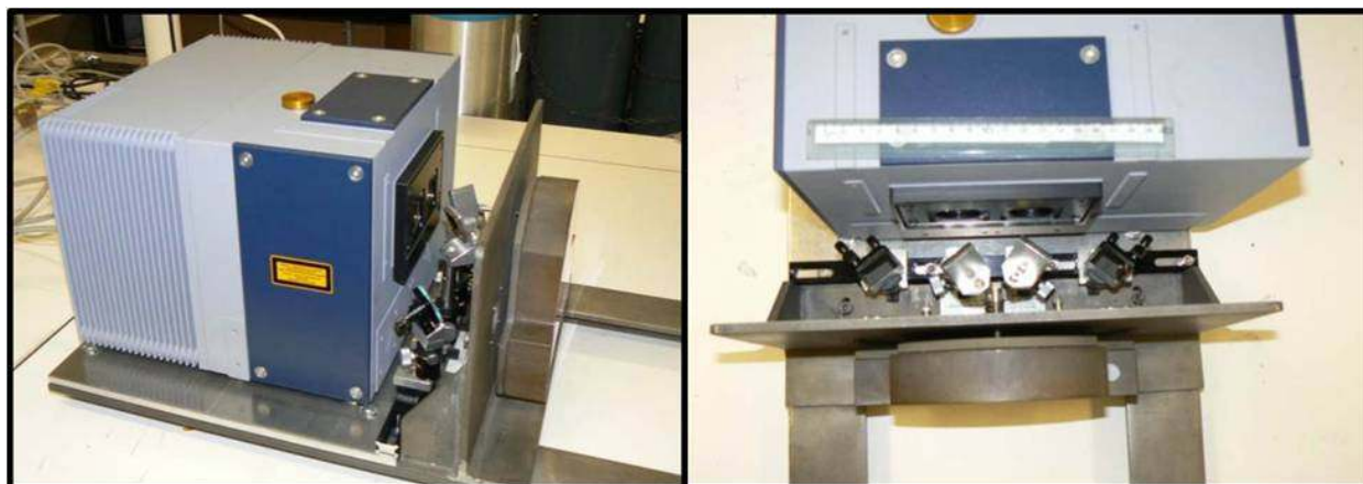
Figure 3.2 FTIR, transfer optics, cell entrance and field mirror. Most of cell is not seen in the photograph. The cell spans the stack ~ 15 m above the fires at the Fire Science Lab as seen in the cartoon of Figure 3.1
