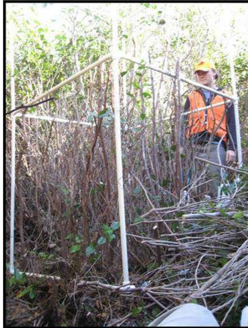
Figure 2.3 Photograph of fuel harvesting at Camp Lejeune for burns conducted at the FSL in Feb. 2009. The harvest shows at typical 1-meter-square plot being harvested for a pocosin sample.
