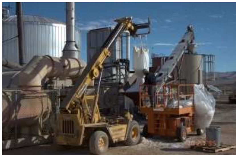
Figure L-3. The salt handling system crushed the salt and transported it to the melter.
