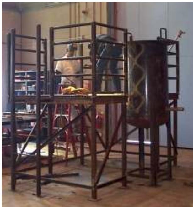
Figure 4-5. Salt recycler used to return spilled salt to the thermal storage system.
