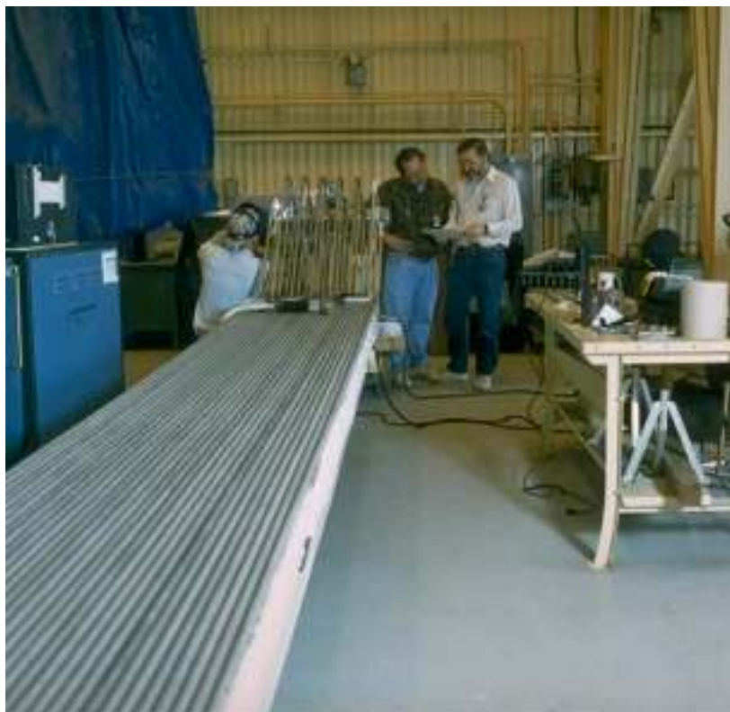
Figure H-11. Single panel from Solar Two receiver. Individual tubes can be seen in the foreground and the headers are in the background. This is before installation vertically into the receiver.
