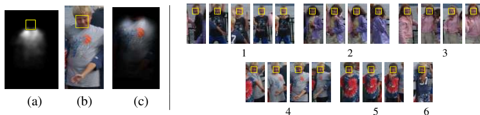
Figure 2: Left: (a) Spatially weighted mask shown relative to a face detection. Brightness indicates weight. This mask is used to weight contributions to a color histogram describing each person’s clothing. (b) Cut out of a person with face detection superimposed. (c) Weight mask superimposed over the image. Right: (1)-(6) The clusters correctly computed for the six different people found in the photos shown in figure 1.
