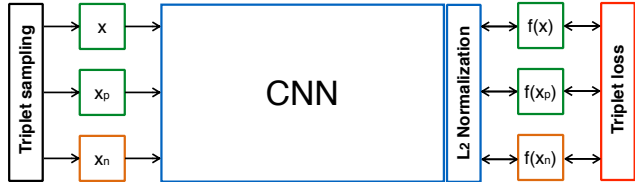
Figure 4. Triplet-based deep metric learning. In the input triplet, image x is closer to x_p than it is to x_n . We train a CNN to preserve this relative ordering under feature embedding f(\cdot) .
