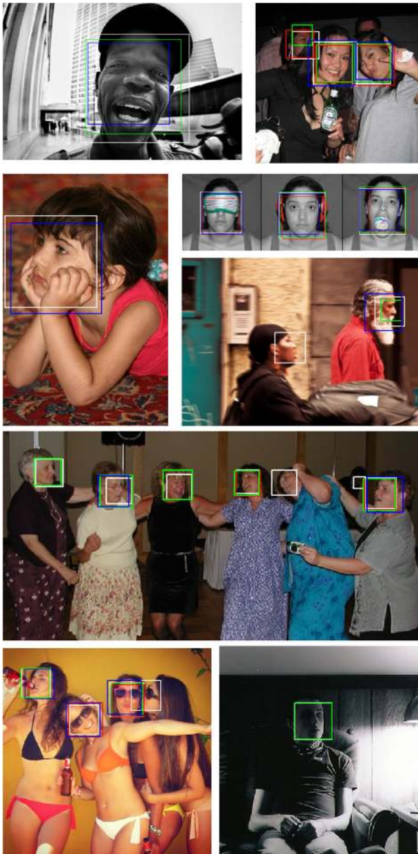
Fig. 5. Ground-truth (white) and detection results of ‘FacePP_v2’ (red), ‘ACF’ (green) and ‘DPM’ (blue) on some test images. Faces without bounding box of specific color are missed by the corresponding algorithm (displayed at a score threshold of 10^{-1} FPPI on the whole test set). Best viewed in color on screen.
