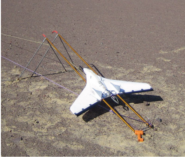
Fig. 3 Photograph of the 1-m wing span DataHawk ready to be launched by a bungee technique. The nearby footprints provide a rough idea of the small size of the aircraft
