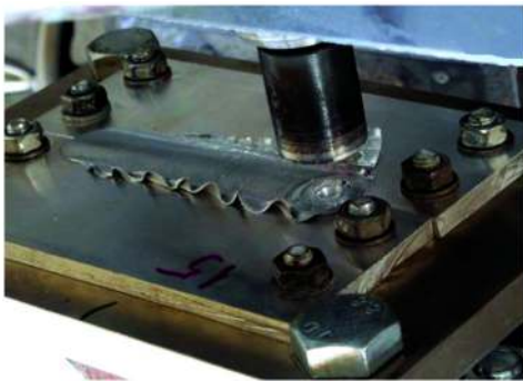
Figure 3. Welded joint with significant amount of flashed material
