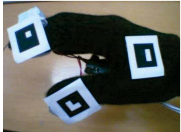
Figure 8: The glove, showing the markers used for hand tracking.
