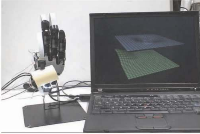
Fig. 1. Example of operation performed by a robotic hand using our finger-shaped sensor. The top and bottom surfaces shown on the laptop display represent surface traction field measured by the sensors mounted on the index finger and the thumb of the robotic hand, respectively.
