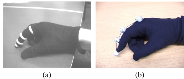
Figure 4. Gloves fitted with retroreflective markers
