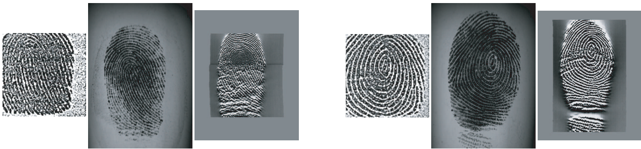
Fig. 2. Example fingerprint images of two fingers acquired with three different sensors (from the BioSec baseline corpus). Fingerprint images of the same finger are shown for a capacitive sensor (left of each subplot), an optical sensor (center) and a thermal sensor (right).
