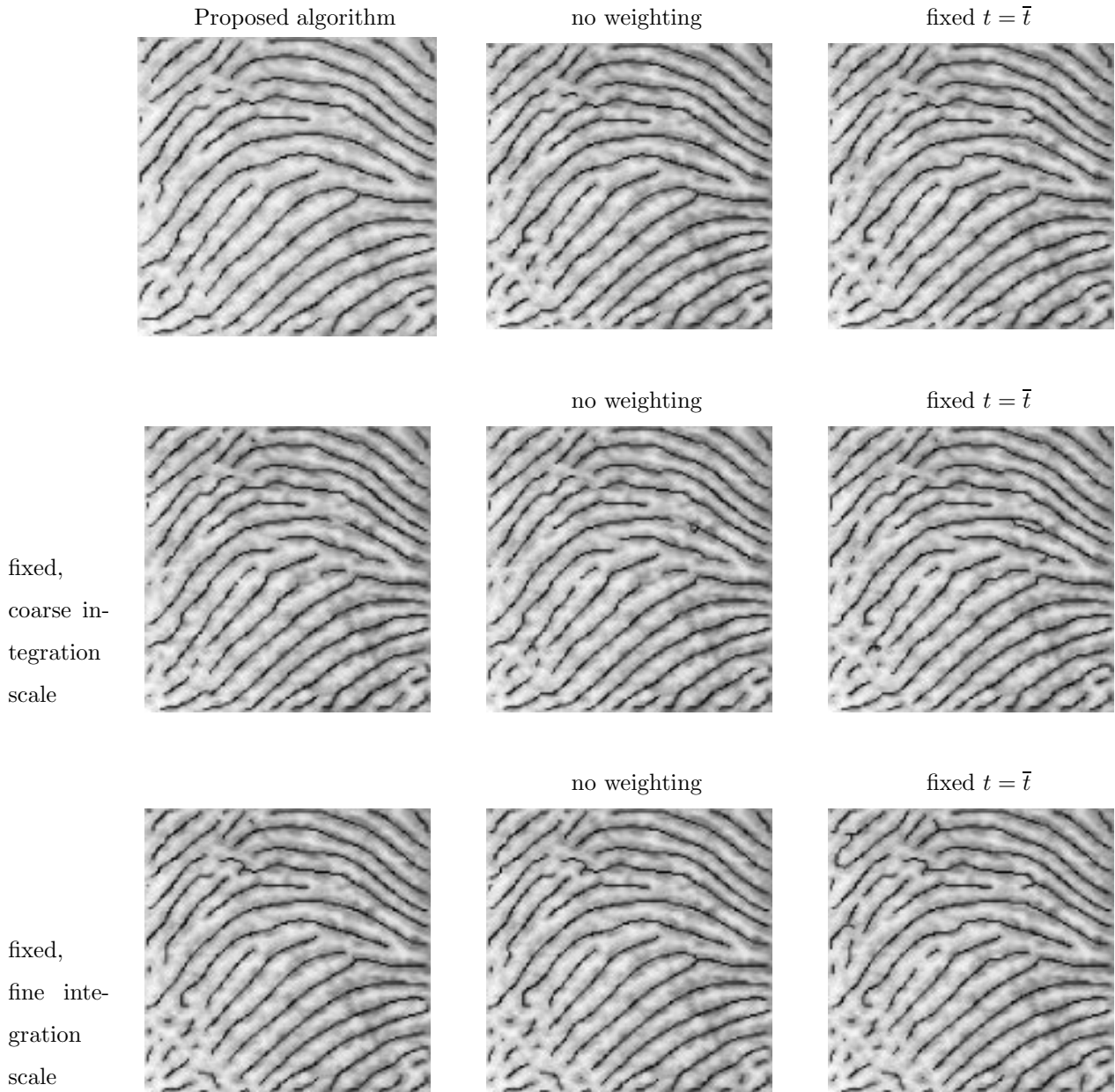
Fig. 3. Illustration of the effects of different modules in the composed shape adaptation and scale selection algorithm. The output of the proposed method (top left) is compared to the result of running the last stage without some of the proposed features. The top row shows the result of applying the last stage with the same local and integration scales as in the proposed method, but without ridgeness-based weighting during shape-adaptation (central column); or with a fixed local scale (right column). The central and bottom rows illustrate the result of using fixed integration scales set to the maximum and minimum values allowed in the proposed algorithm, instead of the proposed scale selection scheme. Observe how the quality of the computed skeleton is rapidly degraded when any of the proposed features is omitted. In particular, observe the ability of the proposed method to spread the correct estimates of the orientation field into the fragmented lower left area, which results in more continuous ridges.
