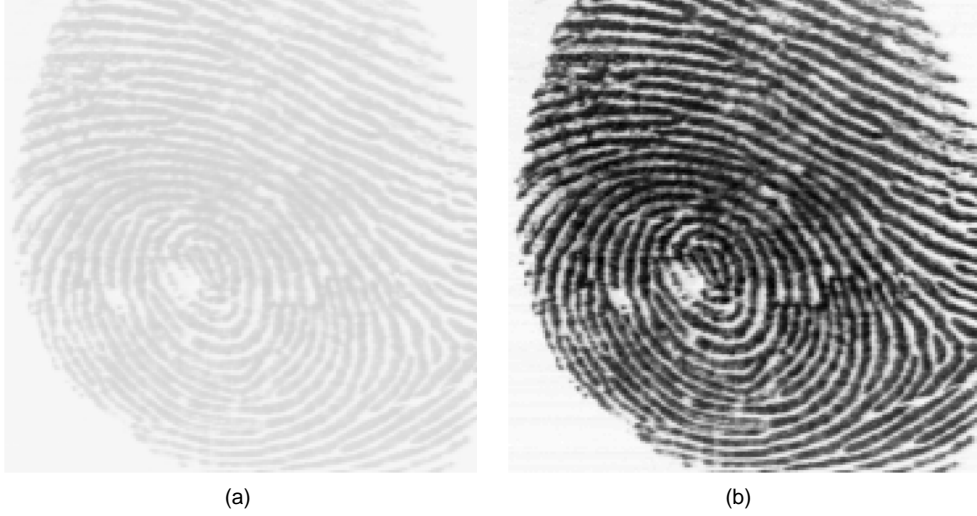
Fig. 6. The result of normalization. (a) Input image. (b) Normalized image ( M_0 = 100 , VAR_0 = 100 ).
