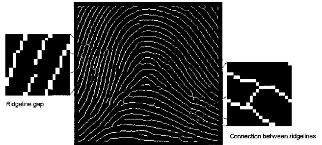
Figure 6. Typical noise in the thinned binary image: false connections between ridgelines (right), and ridgeline gaps (left).
