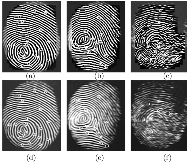
Fig. 4. Sensitivity to the tuning parameters of an enhancement algorithm. Input images are those shown in Figures 3(a-c). Panels (a-c) are obtained using E while panels (d-f) are obtained using E' . Minutiae consistently extracted from both algorithms are considered robust ( \circ ), whereas minutiae detected only by E or E' are non-robust ( \times ).
