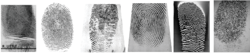
FIGURE 6. Samples of fingerprints from our evaluation database (from left to right: NIST Special Database 27a, CrossMatch Verifier 300 sensor, Digital Persona U.are.U 4000 sensor, FVC2004 optical scanner, FVC2004 thermal sweep scanner, SFinGE fingerprint.)
