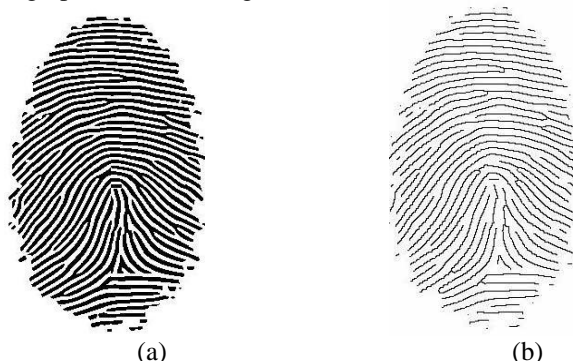
Fig 3: (a) Binarized Fingerprint (b) Image after thinning
