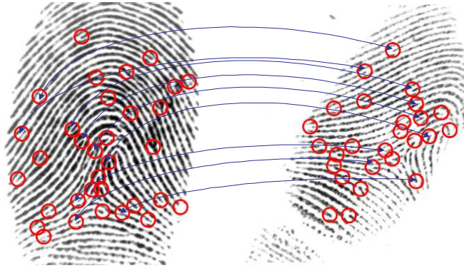
Fig. 2 Illustration of fingerprint intra-class variability. Two different impressions of the same finger with differences in the number and location of minutiae are shown. Among the 33 and 26 minutiae in the left and right images, respectively, only 16 minutiae match and some of these matches are marked.
