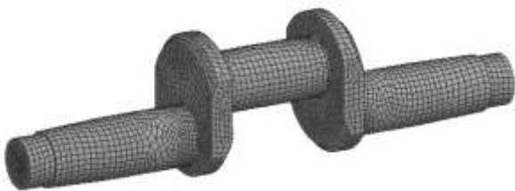
Fig. 4 Meshed model of crankshaft
