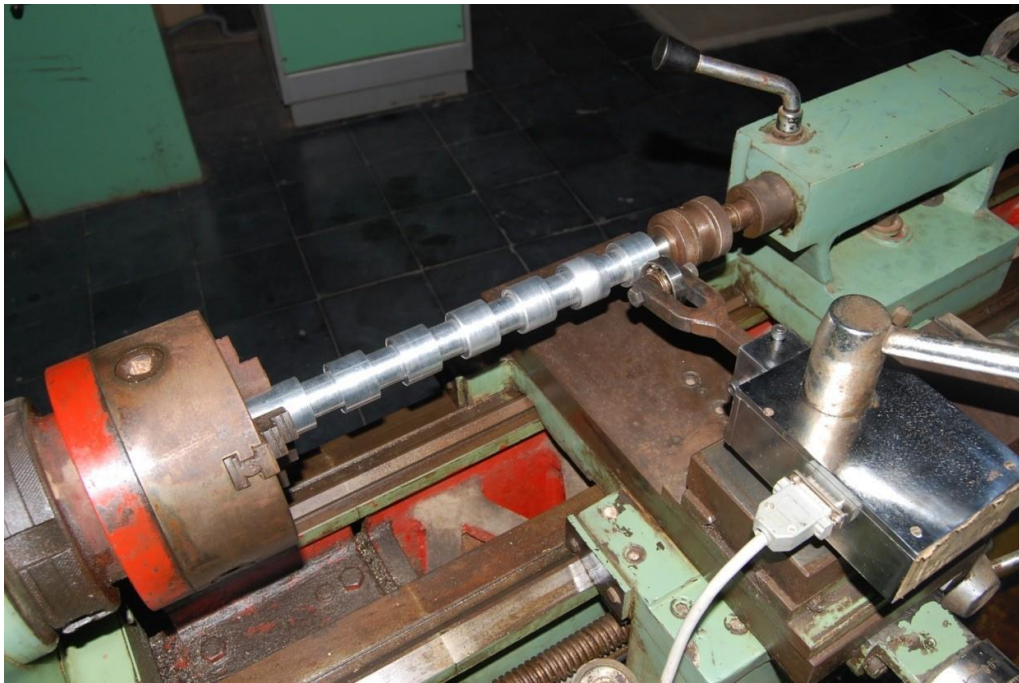
Fig. 9 Photograph showing close up view of aluminum work piece and roller burnishing tool on lathe
