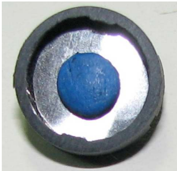
Fig. (5). Piezoelectric buzzer without the front cover. (a) Photo of the buzzer, (b) photo of the buzzer with the mass added on the diaphragm.
