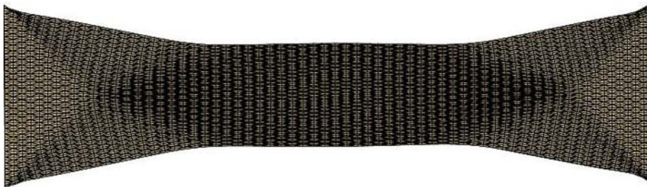
Fig. 17 Different shear zones obtained with a T2-A1 mesh of 40960 elements
