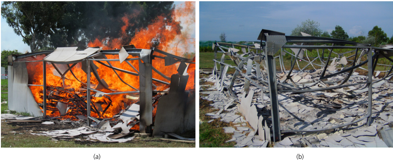
Figure 7. Photographs from full-scale site test: (a) frame collapse; (b) final deformed shape
