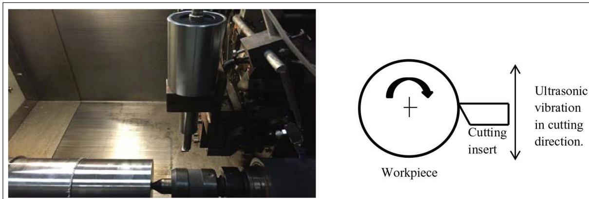
Figure 1. Experimental setup for ultrasonically assisted turning (UAT) experimentation. 31
