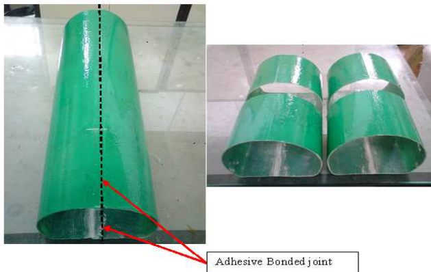
Figure 6. The finished part of composite fuselage section.
