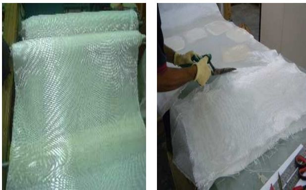
Figure 2. C-glass woven fabric of type 200 g/m 2 .
