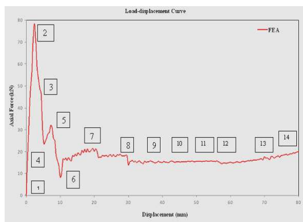
Figure 11. Load-displacement diagram from FEA model.
