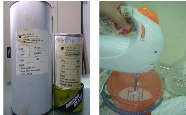
Figure 3. (a) Resin, Hardener and release agent, (b) resin and hardener (4:1) was stirred using an electric stirrer.
