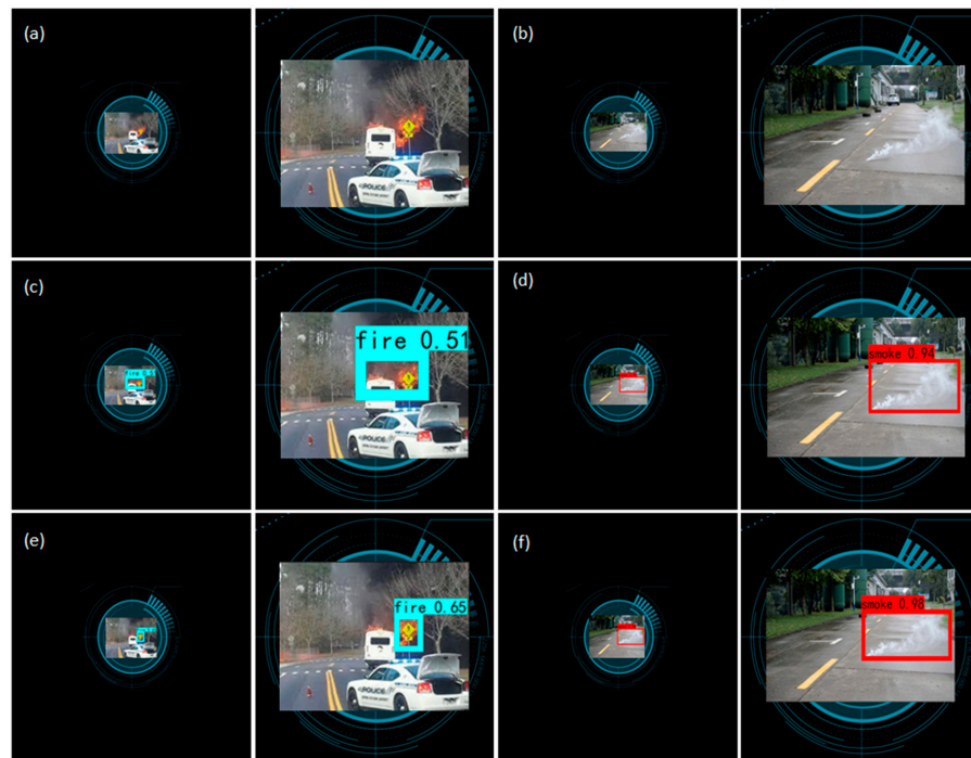
Figure 6. (a,b) Faster R-CNN, (c,d) YOLO-V3, (e,f) Fire-YOLO. The picture shows the results of the Fire-YOLO model proposed in this article and YOLO-V3 and Faster R-CNN to detect very small fire targets.
