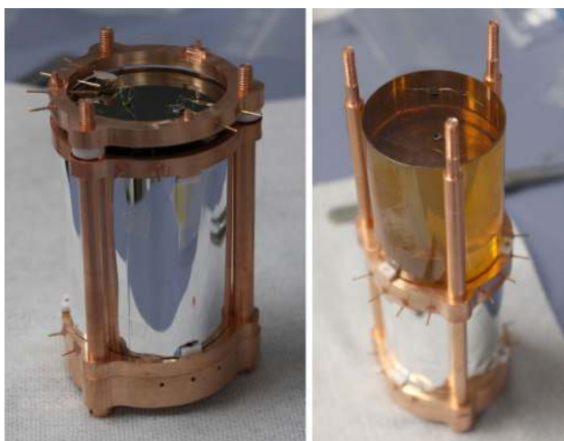
Fig. 2 Two stages of the tower assembly. Left a light detector equipped with an NTD Ge thermistor and a Si Joule heater is mounted on top of a \text{Zn}^{82}\text{Se} bolometer, surrounded by a 3M VM2002 reflecting foil. Right the second \text{Zn}^{82}\text{Se} bolometer is placed on top of the previous light detector
