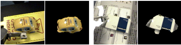
Fig. 7. Challenging segmentations. The example on the right, a blue and white box on a glossy poster, is particularly difficult since it has complex shadows and reflections, but the algorithm successfully distinguishes the white part of the box from the background.
