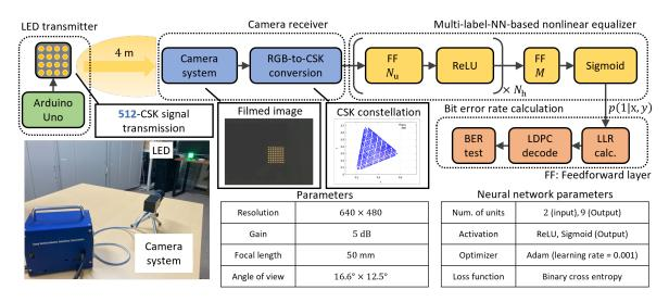
Fig. 2: Receiver configuration and experiment setup.
