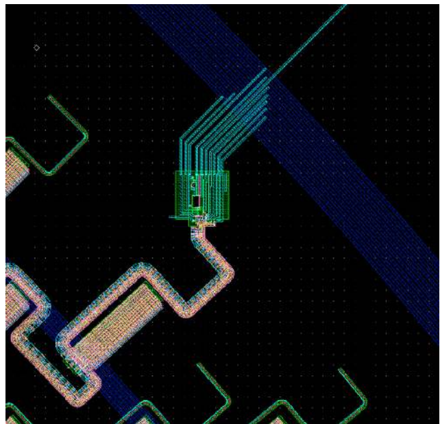
b. Subsection of the prototype mask design illustrating one edge subaperture a serial register, and an output amplifier
