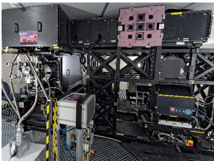
Fig. 11. CIAO: the photograph shows the Coudé room of UT4 in June 2016. The big central structure is the star separator. The CIAO wavefront sensor comprises the tower structure on the left side, with the cryostat connected to a pump on the floor, and the readout electronics located next to it (light gray box connected to blue cooling pipes). The visual wavefront sensor MACAO is located at the lower right.
