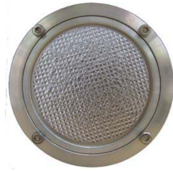
Figure 2. 20 lines per inch Nickel mesh grid filter used as entrance wavelength selection filter of SWAP
