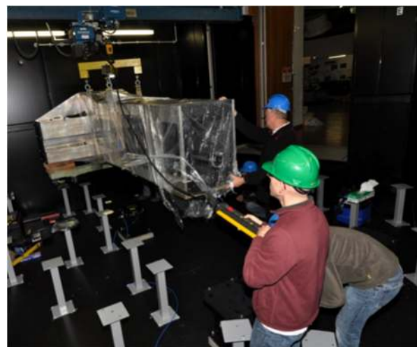
Fig. 1 High Efficiency and Resolution Multi-Element Spectrograph (HERMES) spine being set to air isolators.
