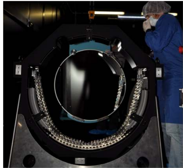
Fig. 4 Collimator mirror being inserted into its chain mount.
