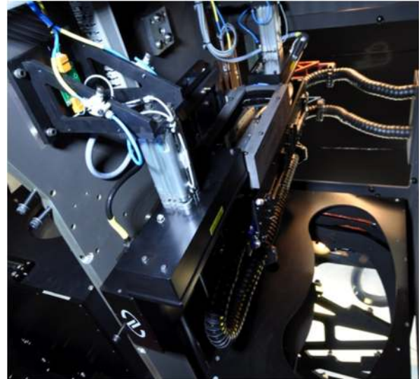
Fig. 8 View of the exchanging slit assembly with the two large fiber cables leading to it and back illuminators positioned directly above it, as well as the corrector lens assembly lens as seen through the kidney-shaped baffle (right).
