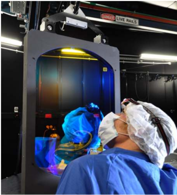
Fig. 10 Beamsplitter being craned into position.
