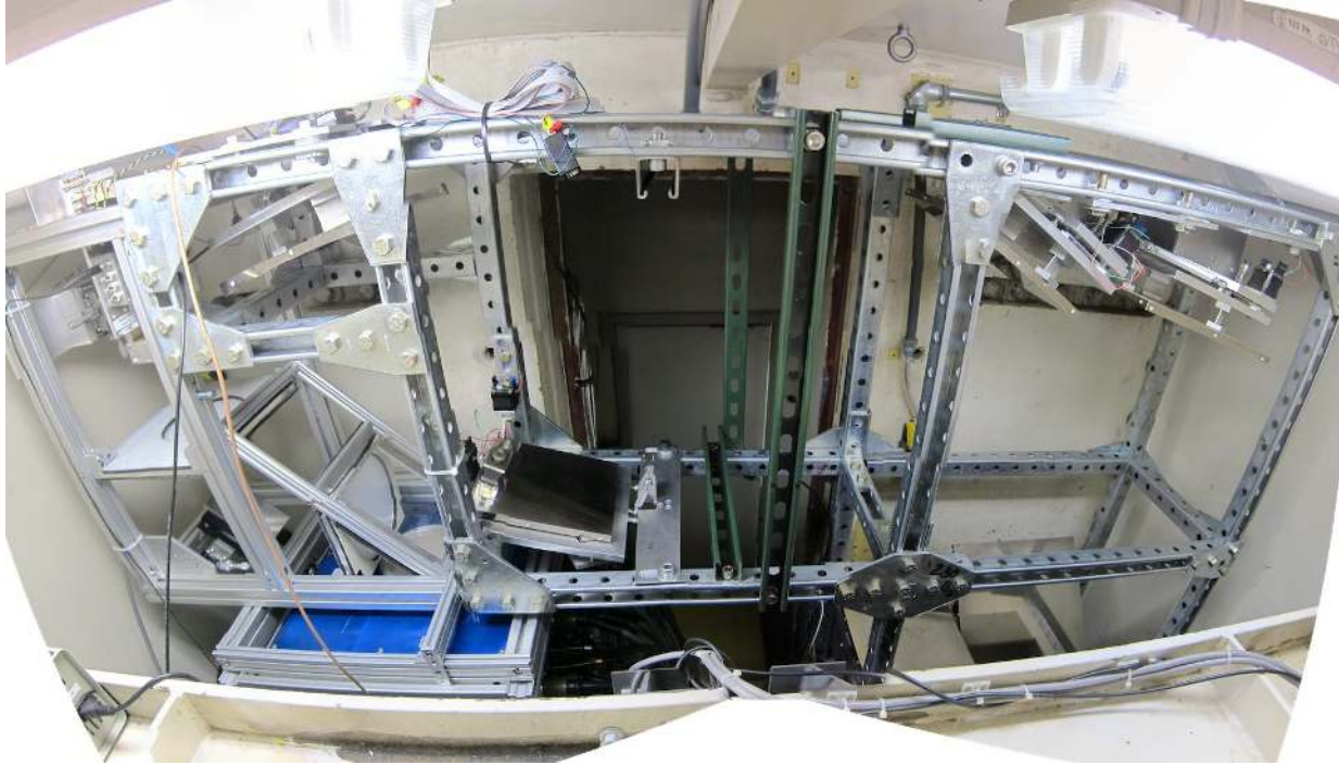
Figure 6. This photograph shows a fisheye panoramic view of SuperCam mounted in the Apex Room of the HHSMT.
