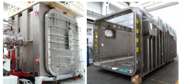
Fig. 7. MITICA beam source vessel under leak test (left) and MITICA beam line vessel under construction (right).
