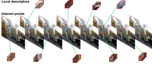
Figure 4. Example local motion descriptors obtained from our video of a person throwing an object to the observer. Locations with salient motion are detected, and their 3-D XYT volume patches are collected as our local descriptors.
