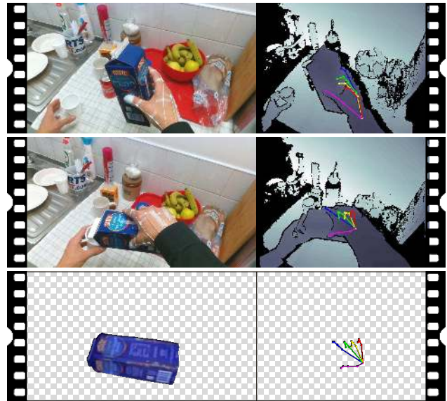
Figure 1: We show two frames from a sequence belonging to the action class ‘pour juice’. We propose a novel first-person action recognition dataset with RGB-D videos and 3D hand pose annotations. We use magnetic sensors and inverse kinematics to capture the hand pose. On the right we see the captured depth image and hand pose. We also captured 6D object pose for a subset of hand-object actions.
