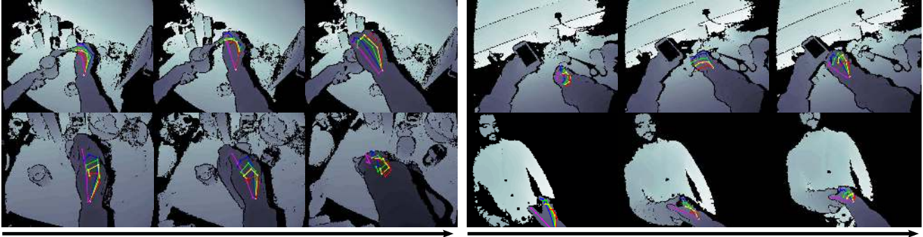
Figure 2: Hand actions: We captured daily hand actions using a RGB-D sensor and used a mo-cap system to annotate hand pose. Left: ‘put sugar’ and ‘pour milk’ (kitchen). Right: ‘charge cell phone’ (office) and ‘handshake’ (social).
