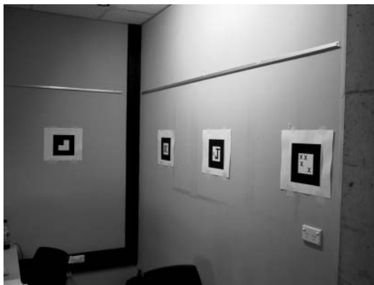
Fig. 10. Fiducial marker on the wall.
