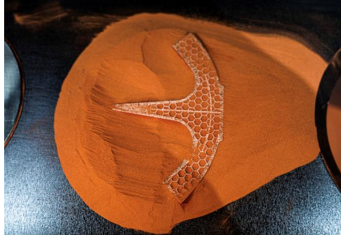
Fig. 4: RFQ proof-of-concept prototype - build job, build plate at bottom position (S.Gruber, Fraunhofer IWS)
